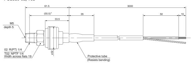
\* Reference dimensions after thread installation
