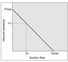
Flow characteristics are expressed in ejector vacuum pressure and suction flow. If suction flow rate changes a change in vacuum pressure will also be expressed. Normally this relationship is expressed in ejector standard use. In graph, Pmax is max. vacuum pressure and Qmax is max. suction flow. The valves are specified according to catalog use. Changes in vacuum pressure are expressed in the below order. 1)When ejector suction port is covered and
