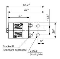
M5 (or M6) (PD port) External release port plug <sup>(1)</sup> <u>M5 (or M6)</u> (P port) Air pressure supply port 10
