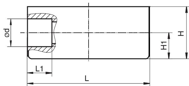
**Union ends with insert - Connection code 7 [mm]**
