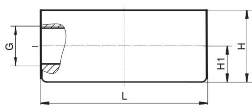
**Solvent cement sockets - Connection code 2; Valve body material: PVC-U (code 1)**
